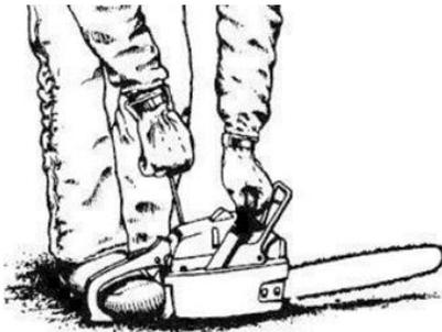
It's always best to start the chainsaw on the ground with the chain brake engaged. Place the right foot inside the rear handle and the left hand firmly on top of the handlebar. Follow the manufacturer's throttle and choke positioning recommendations, pull the starter rope hard, and straight up to start the saw. The starter rope may take several sharp pulls to start the saw when the engine is cold.
