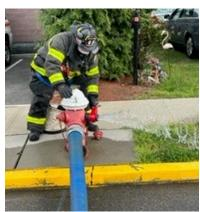
Before disconnection supply hose lines, relieve any residual pressure by using the 4-way valve's relief valve or by opening the  $2\frac{1}{2}$ " gate valve.
