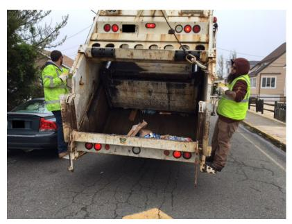
The ANSI standard address the design and construction of the vehicle concerning rider and pedestrian safety by recommending the following: Riding steps should provide a self-cleaning, slipresistant surface that is at least 220 square inches and capable of supporting 500 pounds. The steps should be at least 8 inches deep, mounted behind the rearmost axle of the vehicle, and not more than 24 inches above the road surface.
