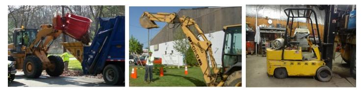
Departments of Public Works use a lot of equipment to lift heavy objects, including forklifts, backhoes, front-end loaders, etc. Workers may need to work near these vehicles when loads are lifted or when the equipment is in the raised position. Points to remember:
