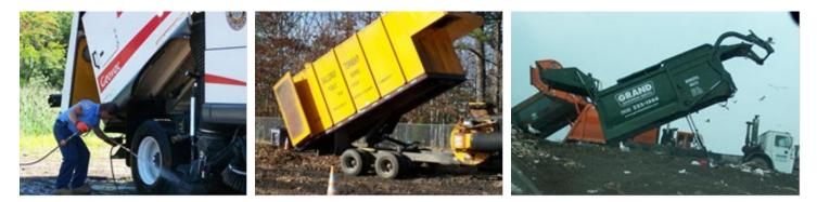
Several pieces of equipment (dump trucks, leaf vacuums, sanitation trucks, and sweepers) have lift gates or bodies that raise. Under normal operations, workers are not permitted to go under a raised component.
